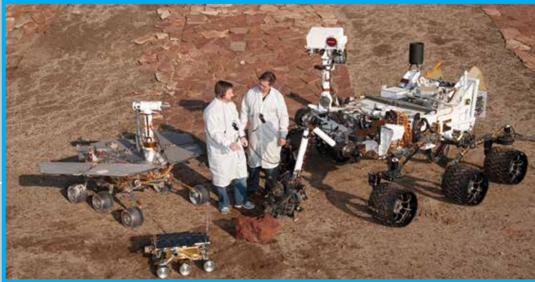
NASA engineers with test models of three different Mars rovers: Sojourner , MER , and Curiosity
